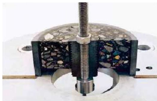
Figure 5-2: Cut view of a CAST specimen at EMPA [source: Poulikakos et al. , 2007]
